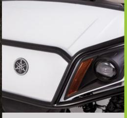
Front brush guard is made of 3/16" steel, 1" round tubing, and 1-1/2" round tubing. Powder-coated for protection.
