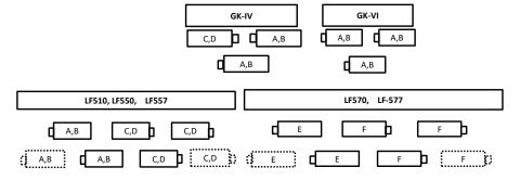
Bi-Directional Groomer/ Brush Use the diagram below to select the correct Bi-Directional Groomer/ Brush part numbers. One option must be selected from each group except "Other" to make a functional groomer or brush system. Note: The Bi-directional groomer / brush system is compatible with the ECLIPSE2 18" and 22" floating head models only. It is not compatible with the ECLIPSE2 18" or 22" fixed head models or the ECLIPSE2 26" models.
