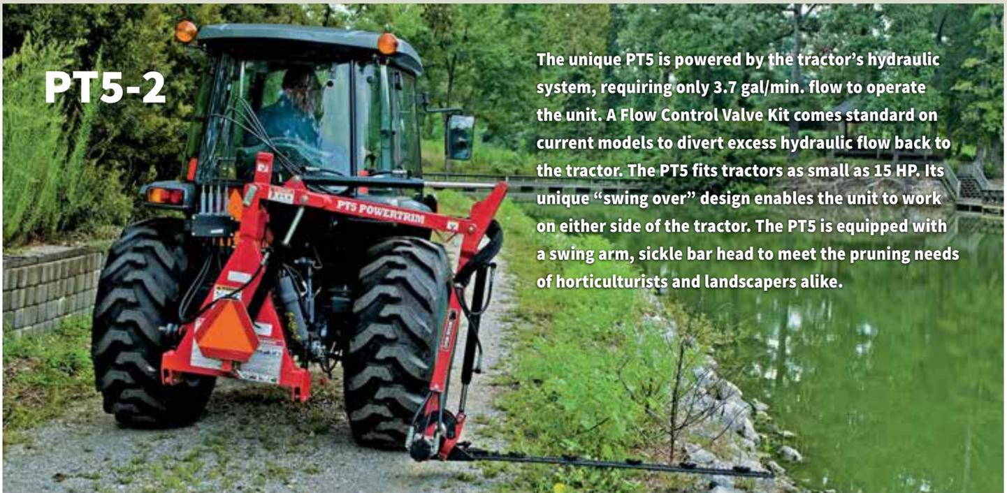
The unique PT5 is powered by the tractor's hydraulic system, requiring only 3.7 gal/min. flow to operate the unit. A Flow Control Valve Kit comes standard on current models to divert excess hydraulic flow back to the tractor. The PT5 fits tractors as small as 15 HP. Its unique "swing over" design enables the unit to work on either side of the tractor. The PT5 is equipped with a swing arm, sickle bar head to meet the pruning needs of horticulturists and landscapers alike.
