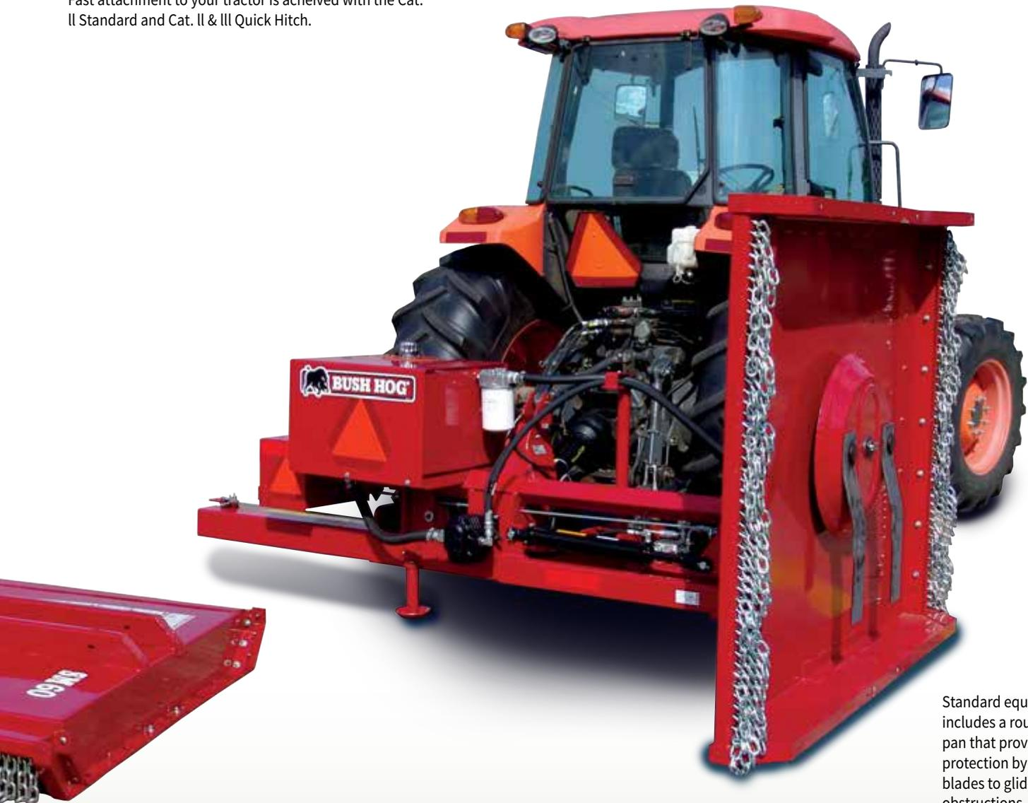
Standard equipment includes a round blade pan that provides driveline protection by allowing the blades to glide over field obstructions.
