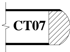
1 1/4" thick top (Internal) Shallow Bullnose Flush
