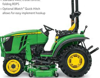
The 2032R and 2038R models offer AutoConnect™ drive-over technology that lets you attach and detach the deck in minutes, all from your seat. Set the height electronically with the industry-leading CommandCut™ that allows for precise and repeatable cutting height.
