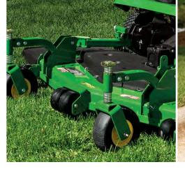
Sweep away. The 60-inch (152 cm) heavy-duty rotary broom can handle light snow, gravel, debris and leaves.
