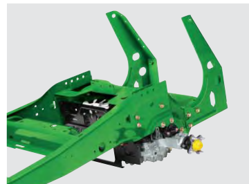
Heavy-duty C-channel frame. Built like a truck, for greater durability.
