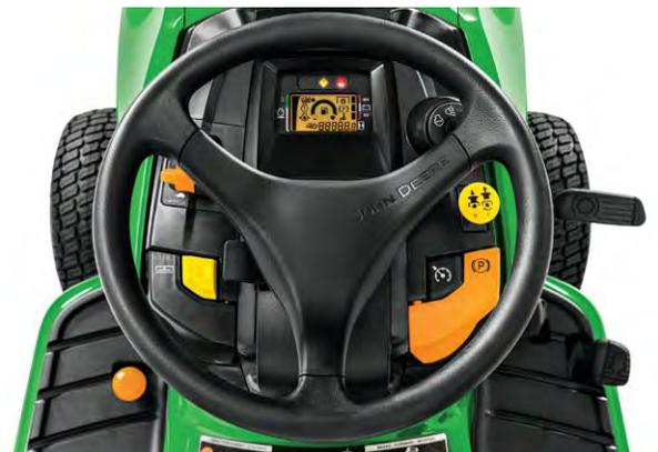
Controls are logically placed, easy to reach, and color coded for easy identification by the operator.
