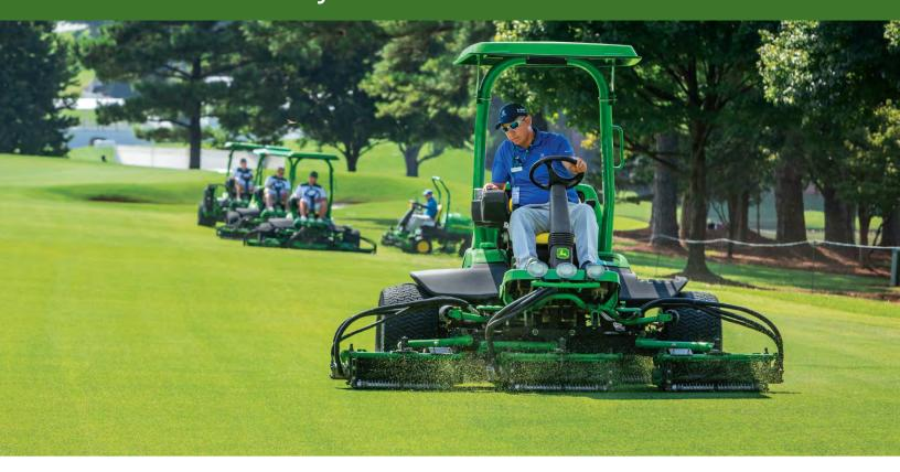
The PrecisionCut™ A Model Fairway Mowers offer several features that separate it from the competition. Like the eHydro™ hydrostatic pump and large capacity motors for serious hill-climbing capabilities. The GRIP All-Wheel Drive Traction System provides superior traction by reducing wheel slip. And exclusive LoadMatch™ lets you cut through wet, lush grass evenly by slowing down the traction speed.
