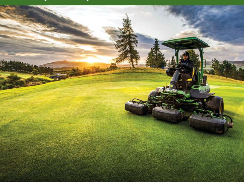
The John Deere E-Cut™ Hybrid Fairway Mowers take highperformance hybrid technology to the next level. The E-Cut™ Hybrid technology uses a 48-V alternator to power the cutting units via electric motors, eliminating all hydraulic leak points from the reel circuit, where 90 percent of all hydraulic leaks occur.
