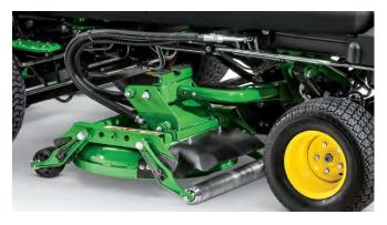
Our unique rear deck design allows for greater clippings dispersion and the deeper shell stands grass up for an even cut.
