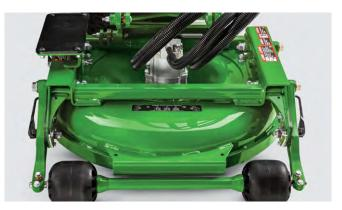
The double yoke on the 9009A means the rotary decks follow the contours in the most undulating terrain for an exceptional quality and consistency of cut.
