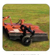
**GUAGE WHEELS** Optional guage wheels guide the mower head over uneven terrain reducing gouging
