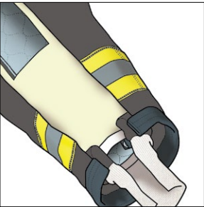
TELESCOPING SLEEVE BAND keeps debris and water out.
