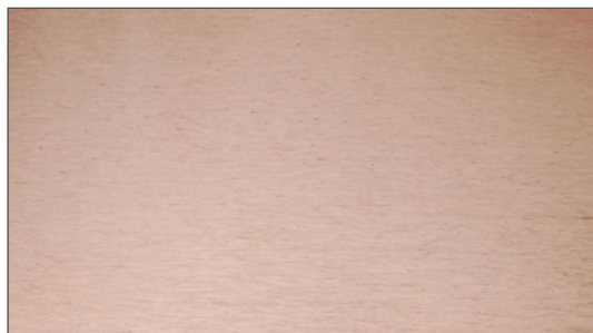
Figure 3.1C. Directionally textured example: C11000, brush finished.
