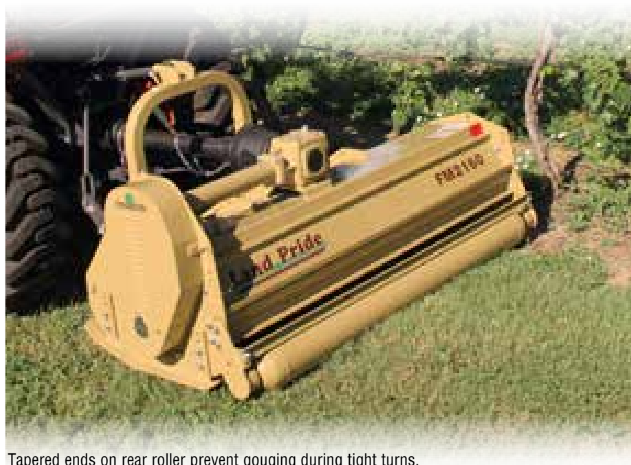
Tapered ends on rear roller prevent gouging during tight turns.
