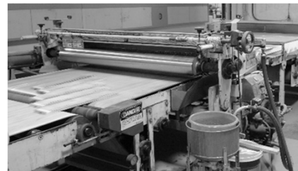
Roll coat applicators apply resin finish
