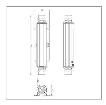
Order Info. 1GSPTK 44-57Vdc(Max 60Vdc)/100W/1000Mbps/10KV Surge Protection/IP67/outdoor use
