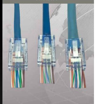
Cat5e Small Cat6 Cat6 Small Cat6A Cat6A Large Cat6 The Smart Feed-RJ45 connectors feature a unique integrated Hi-Lo stagger load bar and allows 'big' conductors to pass through the front end of the connector making it easy to verify the wiring sequence before terminating. These connectors are used with Cat5e/6/6A cabling and is recommended for PoE/PoE+ and Data applications. The termination tool for these connectors is the SFO Crimp Frame and SFO-EX Die.
