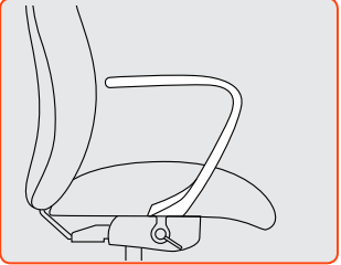
A27 $180 CHROME CANTILEVER ARM Fixed C-shaped arm offers a smooth polished aluminum surface with matching upholstered pad.
