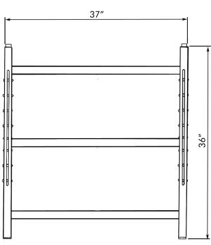
**Bedposts:** 1.5" square steel tubing with 15 gauge (.072") wall thickness.
