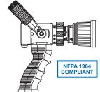
**DQS40P** QUADRAFOG W/GRIP 1" NH (25mm) - Selectable gallonage nozzle with four flow settings of 5, 10, 24, and 40 gpm @ 100 psi (20-40-90-150 l/min @ 7 bar). All lightweight materials, hardcoat anodized aluminum. Flush without shutting down. Quick-change rear valve seat and stainless steel shut-off ball. Pistol grip is mounted below the valve. Rocker lug 1" NH swivel is standard.
