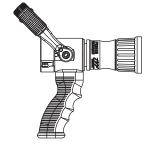
**FS2095P** TWISTER W/GRIP 1.5" NH (38mm) - Dual gallonage nozzle with two flow settings of 20 and 95 gpm @ 100 psi (75 and 360 l/min @ 7bar). All lightweight materials, hardcoat anodized aluminum. Quick-change rear valve seat, stainless steel shut-off ball and a twist "off" position for positive shut off. Pistol grip is mounted below the valve. Rocker lug 1.5" NH (38mm) swivel is standard.
