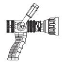
**ME0VPGI-\*\*\*** - METRO 0 W/GRIP1" NH (25mm) - Fixed gallonage nozzle includes flush without shutting down, patented slide-type valve for turbulence-free flow control, six detent flow positions, and "Gasket Grabber" inlet screen. Lightweight hardcoat anodized aluminum for maximum resistance to corrosion and wear. Pistol grip is mounted below the valve. 1" NH (25mm) full-time swivel knurled coupling is standard.
