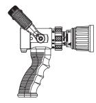
**DQS60P** QUADRAFOG W/GRIP 1" NH (25mm) - Selectable gallonage nozzle with five flow settings of 5, 10, 24, 40 and 60 gpm @ 100 psi (20-40-90-150-230 l/min @ 7 bar). All lightweight materials, hardcoat anodized aluminum. Flush without shutting down. Quick-change rear valve seat and stainless steel shut-off ball. Pistol grip is mounted below the valve. Rocker lug 1" NH swivel is standard.
