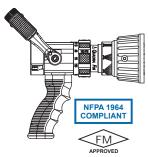
FQS125P QUADRAFOG W/GRIP 1.5" NH (38mm) - Selectable gallonage nozzle with four flow settings of 30, 60, 95, and 125 gpm @ 100 psi (110-230-360-470 l/min @ 7bar). All lightweight materials, hardcoat anodized aluminum. Flush without shutting down. Quickchange rear valve seat and stainless steel shut-off ball. Pistol grip is mounted below the valve. Rocker lug 1.5" NH swivel is standard. FM Approved
