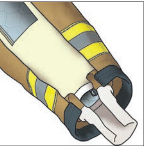
TELESCOPING CUFFS keep debris and water out.
