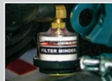
**FILTER MINDER** – Alerts the operator when airflow is restricted in the air canister on dual-element air filters. Available for all models with heavy-duty, remote-mounted, canister-type air cleaners. Standard on 400 and 900 Series. Not available on Kohler-equipped models.
