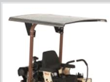
**SUNSHADE CANOPY** – Diamond-plated aluminum or heavy-duty vinyl Sunshade Canopy mounts on ROPS to limit operator exposure to direct sunlight and heat, reduce eye strain and increase operator comfort while providing plenty of headroom.
