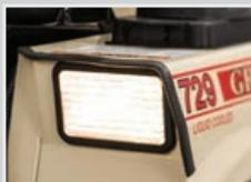
**WORK LIGHTS** – Incandescent standard, halogen or LED optional on 600/700 Series; halogen standard, LED optional on 900 Series. All three work light options available on 200/300/400 Series.
