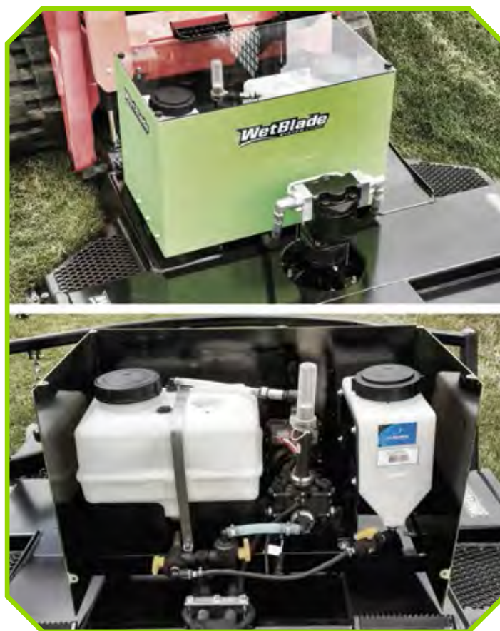
The enclosed WetBlade™ pump system (top) and tanks.
