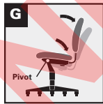
G. Mid-range knee tilt — Pivot point located slightly ahead of center of chair base. Allows user to recline at a slightly more relaxed angle than conventional tilt.
