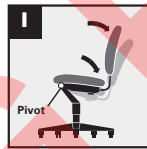
I. Synchronized knee tilt — Back reclines at a 2-to-1 ratio to seat angle. Pivot point located near front edge of chair.
