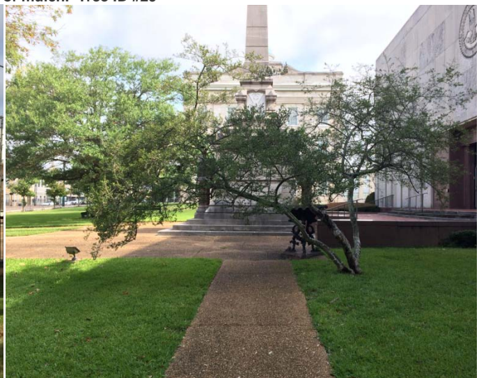
Figure B-10: Example of tree without proper pedestrian clearance. Lowest limb above pedestrian walkway must be no lower than 6'-8".
