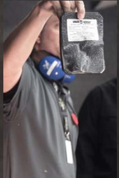
Armor Express VP of Sales & Marketing, Scott Wyatt, holds up the C-Shock concealable special threat plate after it had just defeated two steel core rifle rounds.
