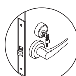
Mortise Lock and Standard Cylinder
