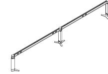
Multiple Hubs with Beam(s) freestanding provide the framework to dock mobile tables. High capacity hubs have additional cutouts to support external electrical and data
