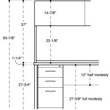
Desk configurations. Attachment hardware is included when ordering a bridge (four splice plates), standard return or Transitional return (two splice plates).
