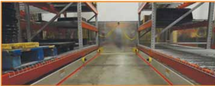
Infrared Floor-Level Beams on Both Sides of the Aisles
