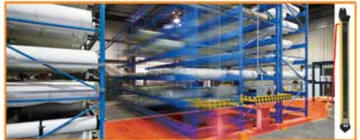
System Entry Infrared Beam Curtain
