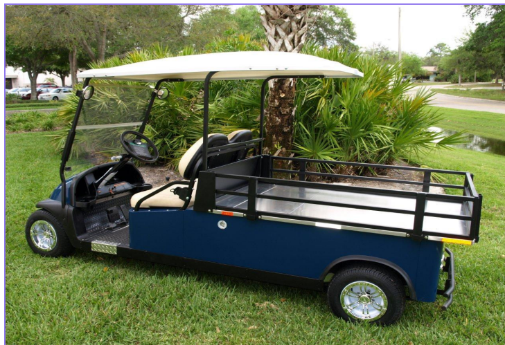
M2SB6 - STAKE BED STYLE UTILITY CART Two Passenger Cart with 6 Foot Stake Bed
