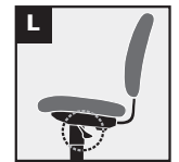
L. Tilt lock — Locks out tilt function when chair is in upright position.
