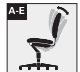
A-E. Back reclines at a 2 to 1 ratio to seat angle. Back angle adjusts independently of seat and can be locked in infinite number of positions within a fixed range.
