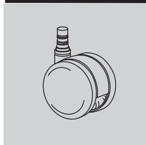
Setu-specific 2 1/2-inch-diameter double-wheel medium roll-resistant caster; black nylon wheels and yoke; soft polyurethane tread; for use on hard floors or carpet; quiet roll technology
