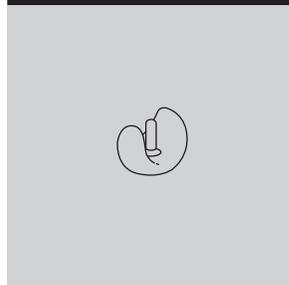
1/4-inch-high, 1-inch diameter glide; thermoplastic CAP material (G1 base has black glides; XT base has clear glides); for use on hard floors or carpet
