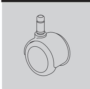
2-inch-diameter soft double-wheel braking caster; black nylon wheels and hood; for use on hard floors only
