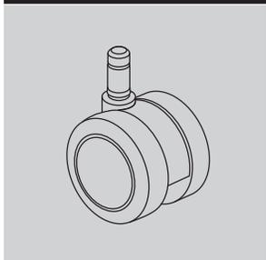
2 1/2-inch-diameter double-wheel caster; black nylon wheels and yoke; soft polyurethane tread; for use on hard floors or carpet
