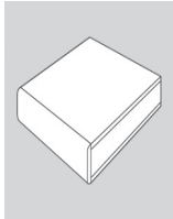
Laminate; 3/8" x 1-1/4" wood band edge; square corner; corner joint is not mitered (34S)
