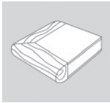
Veneer or laminate; 1-1/4" x 1-1/4" wood bullnose edge; square corner (14S)
