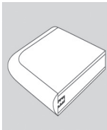
Laminate; 1-1/4" round vinyl bullnose edge; 1-1/2" radius corner (54B)
