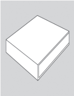
Laminate; 1-1/4" self edge; square corner (64E)
