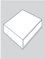
Laminate; 1-1/4" self edge; square corner (64E)
