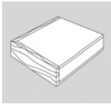
Veneer or laminate; 3/8" x 1-1/4" wood band edge; square corner; corner joint is not mitered (34S)
