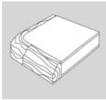
Veneer or laminate; 3/4" x 1-1/4" beveled wood edge; 1-3/4"; radius corner (44R)
