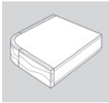
Veneer or laminate; 3/8" x 1-1/4"; 1-3/4" wood band edge; radius corner (34R)
