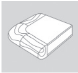
Veneer or laminate; 1-1/4" x 1-1/4" wood bullnose edge; 2-1/2" radius corner (14R)
