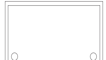
Grommet location for tables 42" or deeper
