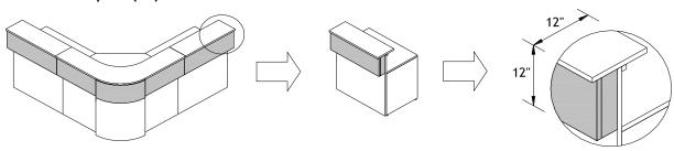
It is possible to add a 12"H vertical panel on the front of the reception, under the transaction shelf. It is in high pressure laminate (HPL).
