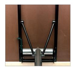
45° struts provide strength to folding mechanism
