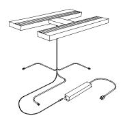
Back-to-back luminaire assembly with arm
