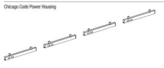
(4) power block assemblies with outlet boxes and face plates
