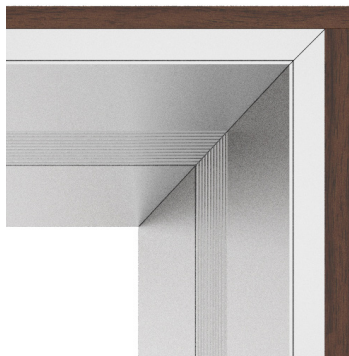
Stealth Team Table aluminum extrusion miter detail
