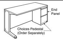
When the 22" (559)-deep Choices Pedestal, 21"/6" (556)-deep Pack Pedestal or 23" (584)-deep Intrinsic Pedestal is used with a 24" (610)-deep work top, the grommet will be unusable. The same is true when using a 28" (711)-deep Choices Pedestal or 27"/6" (708) Pack Pedestal with a 30" (762)-deep work top. On a 30" (762)-deep work top, use an 18"/6" (479), 22" (559)- or 23" (584)-deep pedestal if grommet access is needed.
