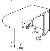
The underside of the work top has predrilled pilot holes to accept Freestanding Flipper Units, Shelf Units, and Screens.
