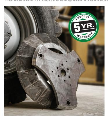
The Diamond proprietary Tri-Hex mulching disc on our rotary heads provides greater inertia in tough conditions, and prevents material build-up between the deck and blade carrier. The disc is constructed of 1" thick 50,000 psi rated steel with hardened, replaceable inserts, giving you unparalleled durability and easy blade maintenance.
