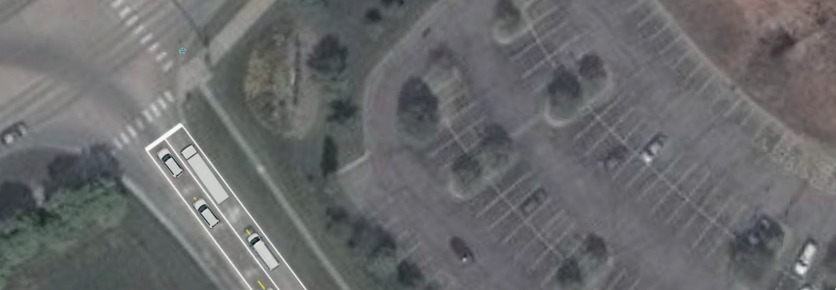
Figure 2. HAWKEYE real-time vehicle classification visualization
