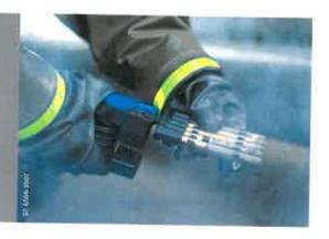
The Dräger CDS civil defense set utilizes colorimetric Dräger detector tubes, the same tube chemistry used by NATO for many years in single tube detectors.
