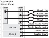
On a split-phase circuit panel, all four circuits are distributed as shown.
