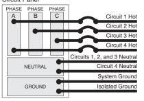
On a single 3-phase circuit panel, all four circuits are distributed as shown.
