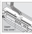
Power and data is maintenance accessible by accessing the power tray on the integrated rail. Devices are then plugged in and the cables are routed through the wire manager to the worksurface. This application is intended for those devices that will remain plugged in and are not managed by users.
