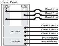
On a split-phase circuit panel, three circuits are distributed as shown
