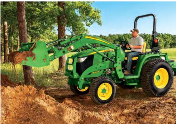
**Quik-Park™ Loaders** - Fast cycle times and impressive lift capacity for superior loading performance. Save time loading and save time putting them on and taking them off on the 3033R, 3039R, and 3046R—a mere three minutes or less.
