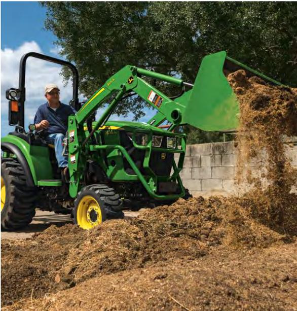
Operator station gives convenient access to loader joystick and hitch lever while independent hydrostatic power steering provides smooth and steady maneuvering, no matter the load.
